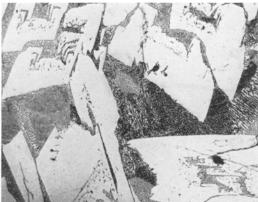
Figure 4 Microstructure of high-Te hypereutectic alloy with 21 wt % As/79 wt % Te. Primary As 2 Te 3 plus eutectic of As 2 Te 3 . Etchant: CrO 3 /Eden (×90).
